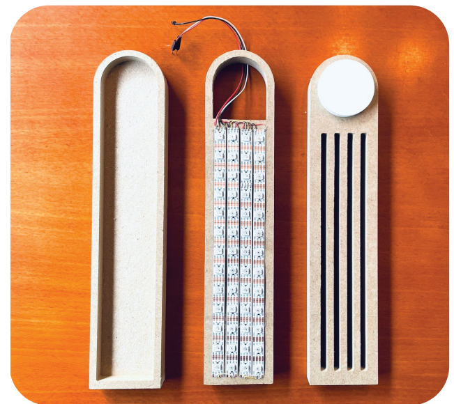
Figure 28. Three bases milled out and the middle covered with LEDs
